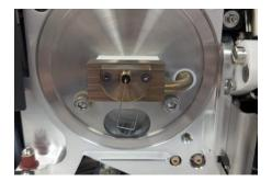
Heater block: The semi-circle shaped piece which is removed by using an Allan key on the two small screws
